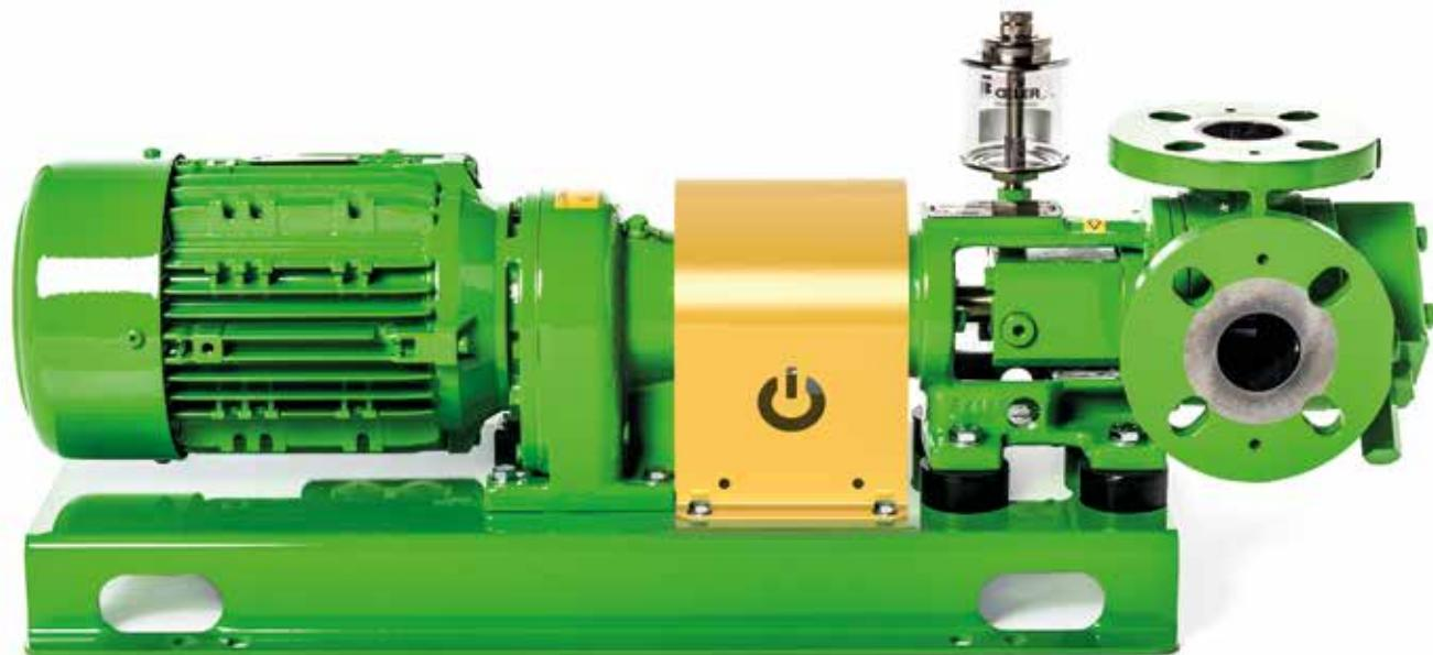
The mechanical seal is protected by a barrier liquid contained in the "quench" which avoids the product to get in contact with the air and to solidify on the faces of the seal.
