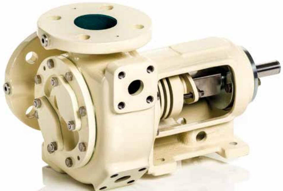
The casing with integrated heating jacket allows to keep the chocolate at a constant temperature and allows to keep the hot water completely separated. The pump is supplied with food compatible materials and a FDA approved packing.
